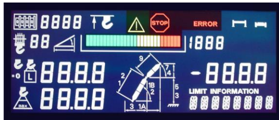
Special displays for crane
